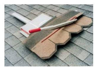
Capable Cutter. Cutting shingles for valleys, rakes, and hips has to be the slowest part of any roofing job, but the *Shingle Shear Model 2003* can speed up the process. This tool has a 20-inch blade and weighs only 16 pounds, making it easy to carry; an adjustable fence helps with repetitive cuts. It sells for \$270 to \$300; replacement blades cost \$25.
