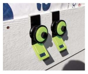
Extra Hands. Handling fiber-cement siding panels by yourself is no small feat. Over the years, I've seen numerous tools designed to make the job easier, but only *SoloSiders* let you tweak the reveal. The devices adjust in <sup>1</sup>/<sub>16</sub>-inch increments from 1<sup>1</sup>/<sub>4</sub> to 1<sup>3</sup>/<sub>4</sub> inches. According to the maker, they won't scratch the siding — and they last a lifetime. A pair sells for \$35.
