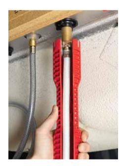
**Super Wrench.** Swapping out faucets and sinks is a mainstay of kitchen and bath remodeling. Ridgid's *Faucet* and *Sink Installer* can help with this job, in several ways. The ergonomically shaped wrench turns 1- and <sup>7</sup>/8-inch faucet and supply-line nuts, frees frozen shut-offs, and secures strainer baskets for installation and removal. It costs about \$25.
