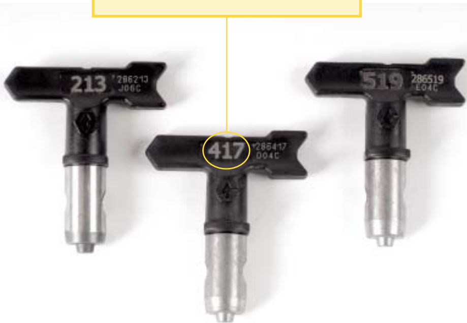
Figure 2. Spray tips come in a range of sizes and are chosen according to the solids content of the paint as well as the fan size needed for the application. Most American manufacturers use a three-digit sizing convention. The first digit equals half the width of the fan; the next two digits represent the orifice diameter in thousandths of an inch.
