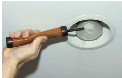
Figure 2. With the blower door running, the author uses a smoke pencil to detect leaks in the house's air boundary. The leaks shown here — at a window sill (above), at a plumbing penetration in a base cabinet (above right), and at one of several can lights (right) — were the result of a kitchen remodel that left the home feeling draftier than before.
