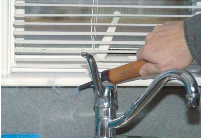
Figure 2. With the blower door running, the author uses a smoke pencil to detect leaks in the house's air boundary. The leaks shown here — at a window sill (above), at a plumbing penetration in a base cabinet (above right), and at one of several can lights (right) — were the result of a kitchen remodel that left the home feeling draftier than before.
