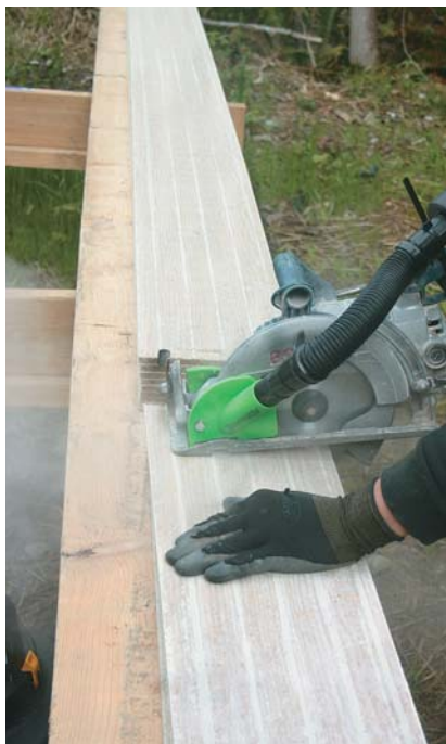
Figure 1. A carpenter cuts first with a Saw Muzzle attached but the vacuum turned off (left). When the vacuum is on, some of the heavier dust falls out the back at the beginning of the cut, but the fine respirable dust is collected (center). With the vacuum on and the blade buried in a stack of siding (right), nearly all of the dust is collected.
