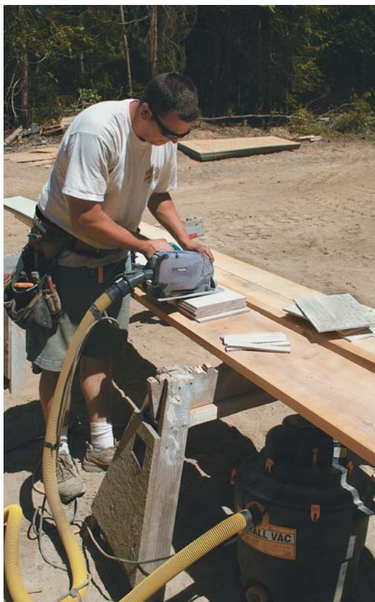
Figure 2. The plastic shroud on the Makita 5057KB makes for effective dust collection when attached to a vac (left). When it's used without a vac, the heavier dust collects in a built-in dust compartment but finer dust escapes (above left). The dust box is emptied through a flip-up lid on back (above right).
