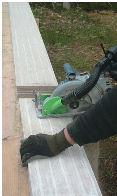
Figure 1. A carpenter cuts first with a Saw Muzzle attached but the vacuum turned off (left). When the vacuum is on, some of the heavier dust falls out the back at the beginning of the cut, but the fine respirable dust is collected (center). With the vacuum on and the blade buried in a stack of siding (right), nearly all of the dust is collected.
