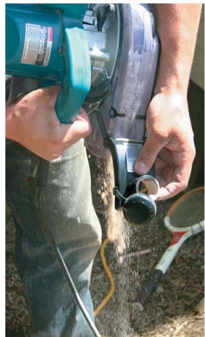
Figure 2. The plastic shroud on the Makita 5057KB makes for effective dust collection when attached to a vac (left). When it's used without a vac, the heavier dust collects in a built-in dust compartment but finer dust escapes (above left). The dust box is emptied through a flip-up lid on back (above right).
