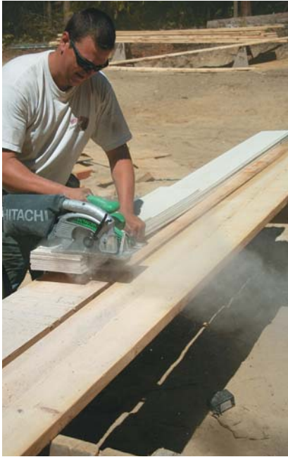
Figure 3. With the dust bag in place, the Hitachi C7YAK allows finer dust to escape (left). Even with a vacuum attached (right), the saw captures less dust than the Makita or the worm drive equipped with a Saw Muzzle.
