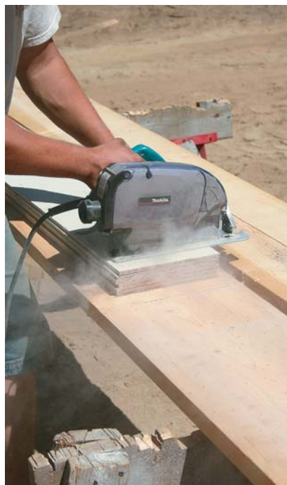
Figure 2. The plastic shroud on the Makita 5057KB makes for effective dust collection when attached to a vac (left). When it's used without a vac, the heavier dust collects in a built-in dust compartment but finer dust escapes (above left). The dust box is emptied through a flip-up lid on back (above right).
