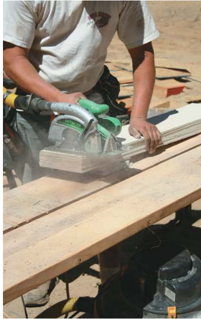
Figure 3. With the dust bag in place, the Hitachi C7YAK allows finer dust to escape (left). Even with a vacuum attached (right), the saw captures less dust than the Makita or the worm drive equipped with a Saw Muzzle.
