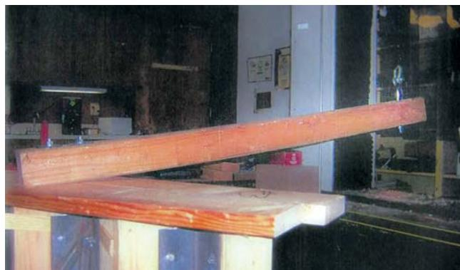
two parallel 2x6 stringers with two  $\frac{3}{8}$ -inch-by-6-inch galvanized bolts inserted through an EZ Stairs bracket (top right) and 2 $\frac{1}{2}$ -inch O.D. malleable steel washers and nuts on the outside of the post (bottom right). Progressively greater loads were applied 42 inches up the post from the tread until the assembly failed. Of three test trials, the lowest point of failure was at 570 pounds; the highest load withstood was 617 pounds.
