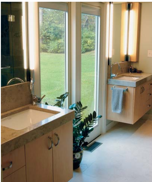
Figure 5. Wall-hung vanities create an open feeling and allow the in-floor heating to run all the way to the exterior wall — decreasing any chance that the plumbing in the cantilever will freeze.
