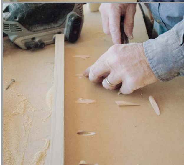
Figure 3. These shelves (top) will be used for shoe storage; their poplar aprons are attached with pocket screws and glue (center). Because the holes would be exposed, the author finishes them with pocket-screw plugs (above).
