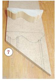
the curved joint. I start with two pieces of MDF the exact width of each piece of molding. The straight template is easy: I trace the profile, then project its flat sections to the edge of the miter as reference points (7).
