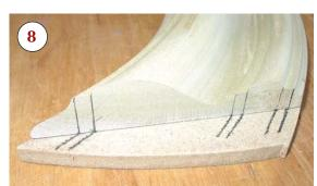
The template for the curved profile is trickier. Because each of the reference points is at a different radius, I shift the piece along the template blank and make a series of dots; connecting the dots gives me reference lines
