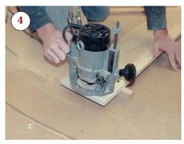
Using a spiral cutter, Junge cuts the ellipse in multiple passes, lowering the bit gradually into the stock — in this case a sheet of MDF. A block of wood screwed to the end of the trammel supports the router above the work (4). Changing the size and shape of the ellipse is simply a matter of moving the pivot points. — *David Frane*
