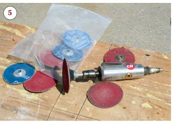
Then I covered the interiors with fiberglass cloth and four coats of resin (4), sanding between coats to smooth outridges and provide tooth for subsequent coats. A pneumatic die grinder with a flexible sanding pad (5) works great for this task. I found that the fiberglass resin dries in 30 minutes or less, depending on the temperature and humidity. I also sanded the top coat, to help the trowel-on tile water-proofing membrane adhere.
