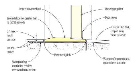
resemble a shower pan, with upturned walls and the upturned membrane flashed and sealed at the threshold to prevent wicking.
