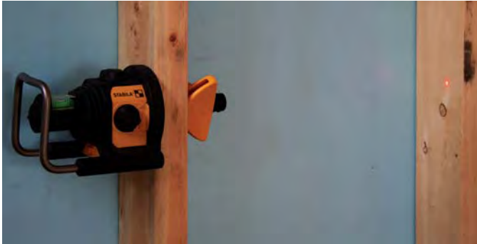
Figure 2. A hole-locating laser makes it easy to drill a series of perfectly aligned holes. It's attached to the framing member through the first hole and projects the location of the next hole onto the adjacent joist or stud. With the on-board vial, the holes can be sloped \frac{1}{4} inch per foot for DWV piping.
