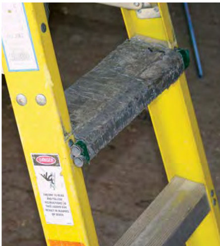
Figure 4. The conduit is generally cut with a hacksaw or cordless recip saw (right). A pair of conduit scraps duct-taped to a rung on the ladder help hold the pipe at a comfortable level (below). Once it's cut, the inside is reamed (below right) so that the burr edge doesn't cut or chafe the insulation when the wire is pulled.
