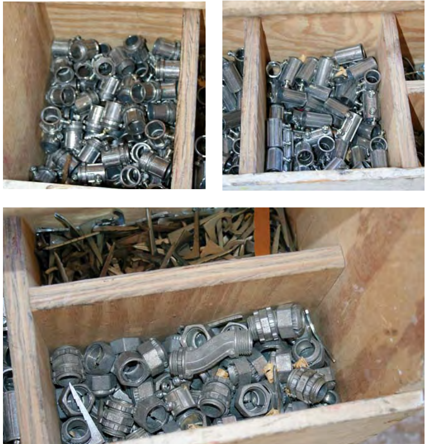
Figure 6. Most conduit runs are made with just a few fittings. Among the most common are the pipe-to-box connectors used to terminate the pipe at the work box (top left), couplings for joining sections of tubing (top right), and "Jakes" for very tight offsets (above).
