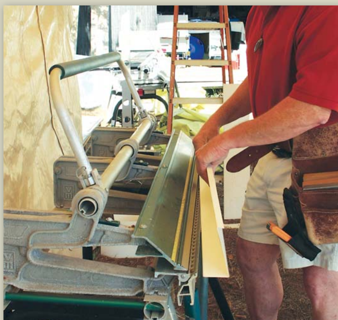
Figure 1. After bending a short lip on the back of the vinyl coil stock, the author uses 4 9 / 16 -inch gauge blocks (far left) to quickly position the material for a second bend (center). Because vinyl springs back, the corners must be slightly over-bent (left).
