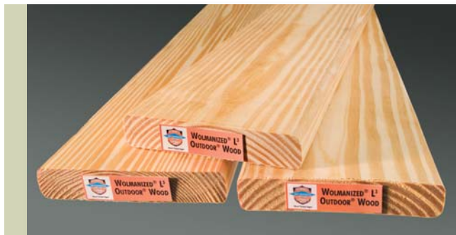
Figure 7. Intended for aboveground use, the non-metallic Wolmanized L3 wood has been evaluated by the International Code Council and is listed in the AWPA Book of Standards . The company adds a pigment to its formula to distinguish its light brown treated lumber from other types of treated lumber. It is backed by a lifetime limited warranty.
