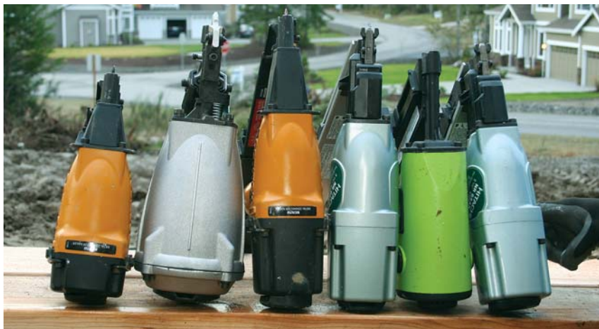
Figure 2. Hardware nailers come in a range of sizes (top). The ones with short magazines are compact and maneuverable but require frequent reloading. The MCN150 (far left in above photo) was the shortest tested. The Paslode (second from left) has the widest housing.
