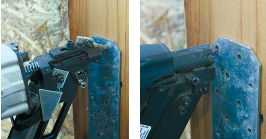
Figure 1. Paslode's gun has a probe (left) that the operator uses to align the nail with the hole in the hardware; it pivots out of the way when the gun is fired. With other guns, the nail itself can be placed directly in the hole (right).
