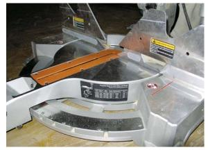
laser-etched onto a high-contrast stain-less-steel plate. On the fence is an erasable writing surface for marking repetitive cuts; on the base, a pair of tables for cutting crown on the flat.
