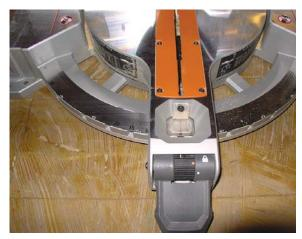
Miter and bevel settings are adjusted with large paddles. The miter lock has a thumb-wheel for engaging and overriding detents. The author found both miter and bevel settings to be accurate right out of the box.
