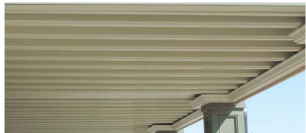
UnderDeck's vinyl panels arch between the joists and drain to troughs that run the length of the joists into a gutter.
