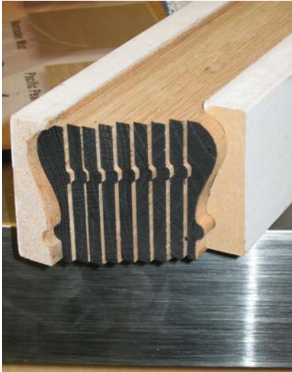
Figure 1. Bending rail is made up of interlocking pieces of wood that join to form the profile of a solid handrail. The outer pieces are bending molds — which are used during glue-up to protect the rail and provide flat clamping surfaces.
