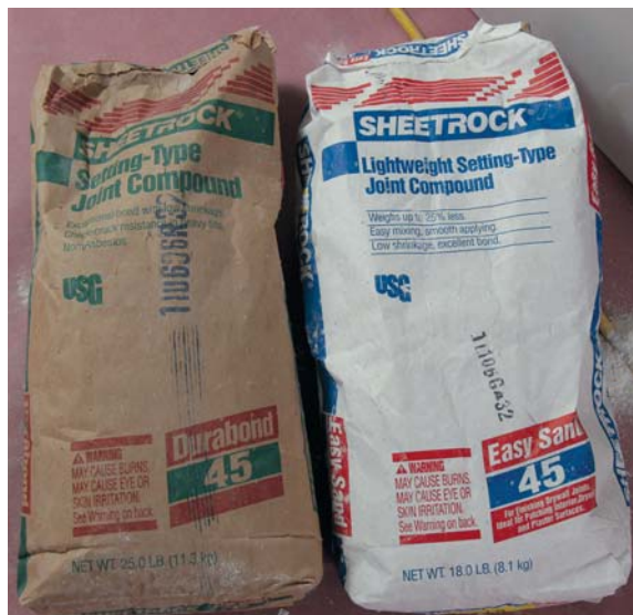
Figure 1. Though not as hard or as strong as regular setting compounds (at left), lightweight setting compounds (at right) are sandable and almost as easy to finish as premixed joint compounds.
