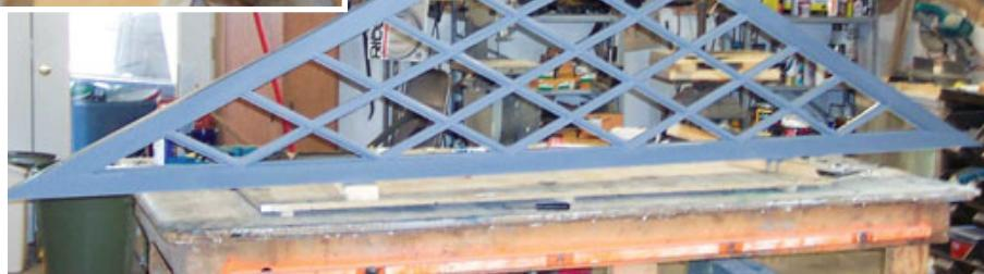
10-foot-wide window's outside dimensions on a sheet of plywood, then milled the parts from clear pine stock with cope-and-stick shaper cutters.
