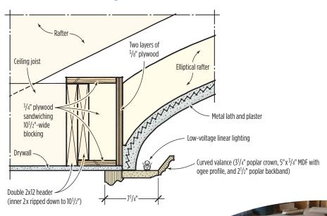
10<sup>1</sup>/2 inches, on all eight sides. The step-up created by the narrower framing members would accept a <sup>3</sup>/4-inch plywood ring that would turn the octagon into an accurate circle (2). Nailed to the bottom of the 10<sup>1</sup>/2-inch members, the plywood would be flush with the bottom of the joists. A second plywood ring would go on top, sandwiching short sections of blocking to create a sturdy platform to support the dome rafters.
