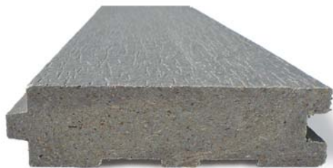
Figure 2. Correct-Porch solid T&G planks are intended for use on covered porches with sloped floors. A built-in spacer "bead" creates a small gap between planks that allows for drainage and thermal expansion. The composite can be painted or left unfinished.
