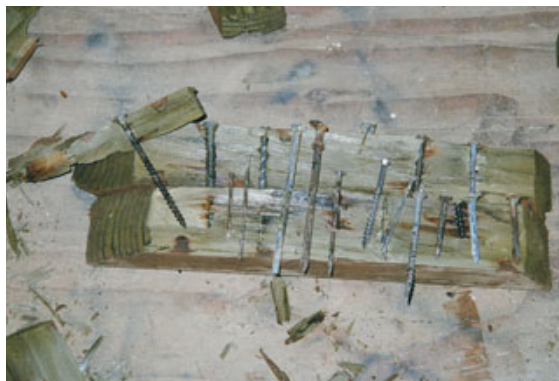
Figure 2. After one year's outdoor exposure in Olympia, Wash., galvanized fasteners driven into ACQ-treated lumber have begun to corrode (top left). After five years in the same environment (bottom left), rust is apparent everywhere.
