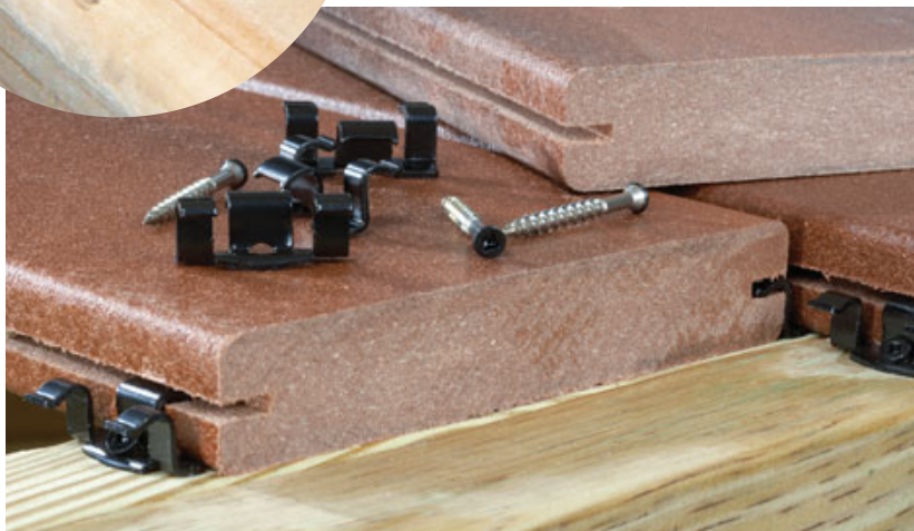
Figure 5. Hidden-fastener clips usually have either prongs that are driven into the side of the deck board (inset) or tabs that engage in grooves milled in the side of the decking (above).
