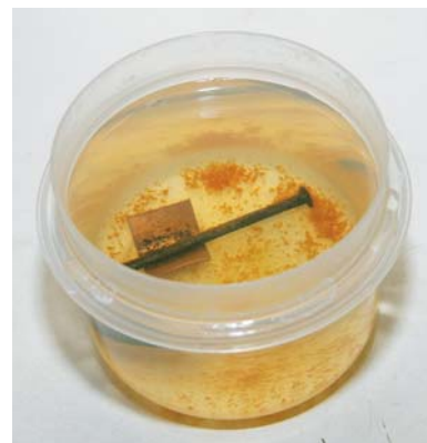
Figure 2. In the presence of an electrolyte, the copper in treated wood chemically attacks steel. This nail was bright and shiny when placed in a salt solution with a piece of copper. Twenty four hours later, the water is tinted and rust has settled to the bottom of the container.
