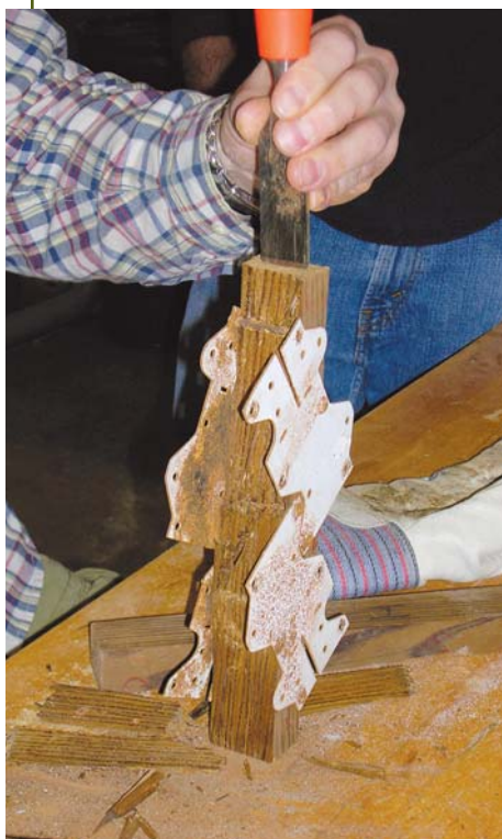
Figure 8. Trust the hardware manufacturer, not the wood treater, to provide information on whether a product will work with a particular preservative. Hardware manufacturers continually perform accelerated weathering tests to ensure durability.
