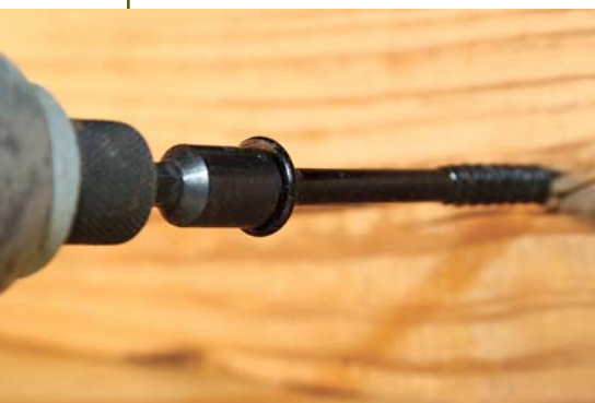
Figure 7. The new generation of thinner ledger screws gain their strength from heat treatment. Hot-dip galvanization would negate this, so most such screws are polymer coated.
