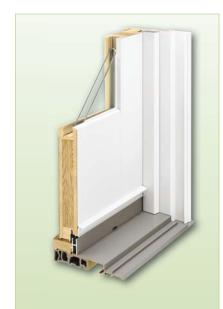
Andersen's 400 Series patio doors are built the way many wood doors are, with LVL stiles and rails. Instead of being finished with wood veneers, though, the LVL is wrapped with phenolic that is glued and pressed into place.
