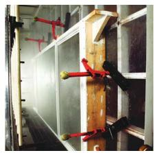
To earn AAMA or WDMA certification, window and door samples are tested for their ability to resist wind (far left) and water (left). For approval in high-wind zones, windows and doors need to be able to withstand a 4-foot-long 2x4 shot out of a cannon at 27 mph (for Wind Zone 3) or an 8-footlong 2x4 shot out of a cannon at about 34 mph (for Wind Zone 4). Below, a test in progress.
