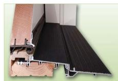
Jeld-Wen's inswinging-patio-door sill has a treated pine subsill, an adjustable vertical-grain Douglas fir threshold, and an anodized aluminum extrusion. The sill is fitted with a 2-inch extension to fit a  $6^9$ /16-inch-thick wall.
