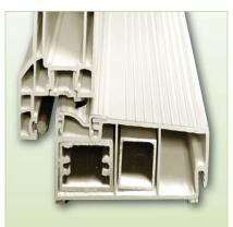
The sills of Gorell's vinyl patio doors are cut from the same aluminum-reinforced extrusions as the jambs. At the corners, the extrusions are mitered and heatwelded together like a picture frame, creating a waterproof joint.
