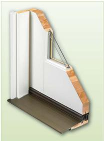
The vinyl cladding on Peachtree's 300 series door won't corrode in a marine environment — an advantage over aluminum. Also, vinyl can be heat-welded, for watertight joints. However, it becomes brittle in the cold and tends to degrade with UV exposure.
