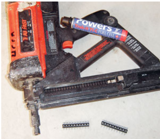
Figure 7. A TrakFast gas-powered nailer can outshoot a PAT in many applications, and it handles pins up to 1 1/2 inches long. The author's crew relies heavily on this tool when fastening bottom tracks to the floor.
