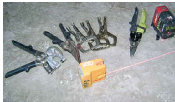
Figure 5. A fundamental tool collection covers most steel framing tasks.
