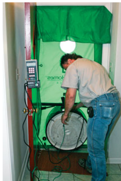
Figure 7. The technician verifies the correct operation of a new furnace and water heater (left) and documents the safety of the new kitchen range (below left). A final blower-door test (below) indicates the increase in house airtightness, from 3,600 CFM-50 to just over 1,900 CFM-50.
