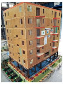
To find out whether tall wood-framed buildings can be designed to withstand seismic activity, researchers recently tested a seven-floor condo tower on Japan's E-Defense shake table (above). The building was reinforced with an anchored tie-down system connected to steel special moment frames on the ground floor (above right), but otherwise was built using standard construction materials and techniques. Large hydraulic pistons provided the thrust to simulate a magnitude 7.5 earthquake (right).
