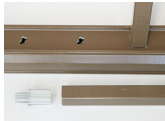
Figure 4. The hollow balusters in GAF's RailWays system fit over ribbed plastic fittings screwed to the rail before assembly (above left). Fibron's Horizon Plus Railing (above) relies on press-fit plastic inserts — one end fits in the baluster and the other in a slot in the rail. The balusters in Trex's Artisan Series (left) drop into routed openings in a vinyl spacer strip; it snaps into the rail.
