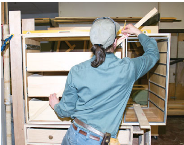
Figure 5. It's faster to install drawer hardware before the cabinet is assembled; a simple mounting jig helps ensure accuracy (top left). The boxes are screwed together without glue, making assembly reversible (top right). The masts at the side of the assembly bench hold the cabinet square as drawers are adjusted and the backs are tacked on (left). The post is screwed to one cabinet, and the adjacent cabinet is notched to tuck in behind it (above).
