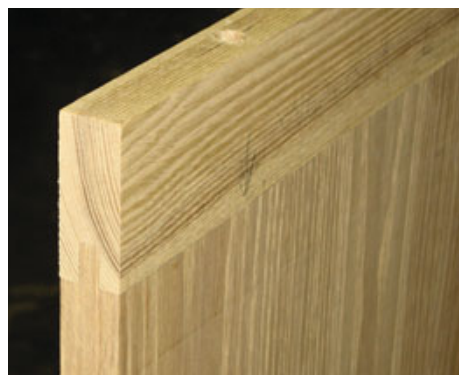
Figure 4. To avoid cross-grain shrinkage problems on bread-board doors, only the middle section of the crosspiece is glued; screws are used at the outer ends. Oversizing the countersink holes allows the screws to flex slightly, accommodating expansion of the door panel.
