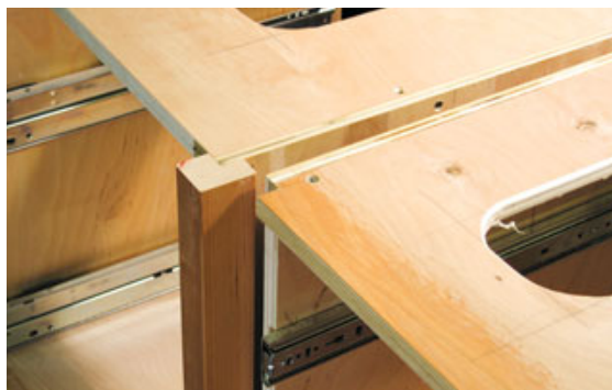
Figure 5. It's faster to install drawer hardware before the cabinet is assembled; a simple mounting jig helps ensure accuracy (top left). The boxes are screwed together without glue, making assembly reversible (top right). The masts at the side of the assembly bench hold the cabinet square as drawers are adjusted and the backs are tacked on (left). The post is screwed to one cabinet, and the adjacent cabinet is notched to tuck in behind it (above).
