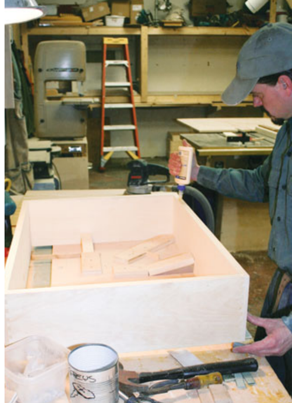
Figure 3. For fast drawer production, the author keeps a workstation set up with a router and dovetail jig for making parts (far left) and a simple squaring jig for assembly (left). He also uses Blum's Metabox system, which is ideal for site-built drawers because it requires only a plywood bottom and a finished front (above).
