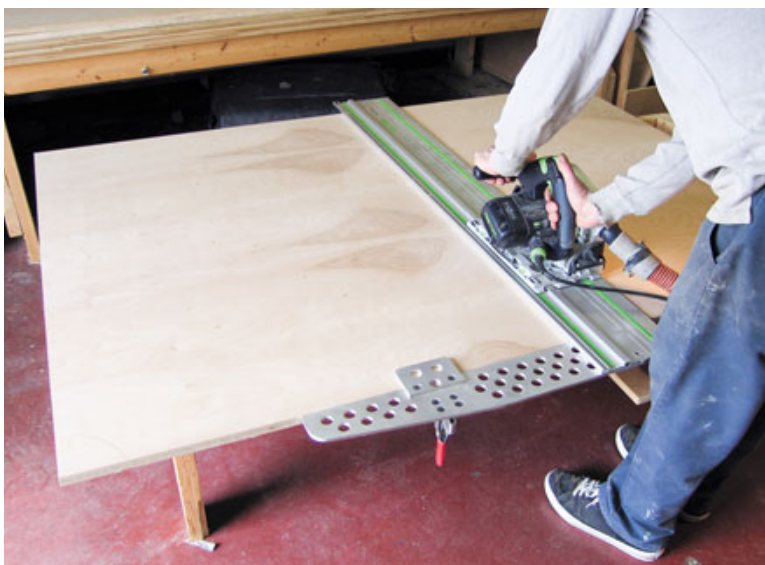
Figure 2. The author uses a Festool track saw to cut plywood cabinet parts. A custom T-square fitting allows for accurate crosscuts (above). A dedicated router is set up to cut \frac{1}{4} -inch-by- \frac{3}{4} -inch rabbets for carcase corner joints (top right). A hardwood gauge block makes quick work of setting the fence and blade height for rabbetting the posts (right).
