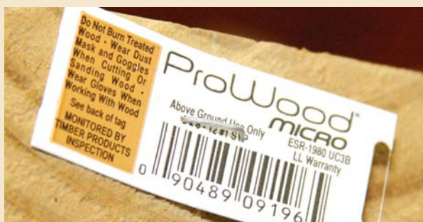
Treated-wood end tags identify the brand of lumber, provide an evaluation service report number, and specify Above Ground, Ground Contact, or other permitted uses.
