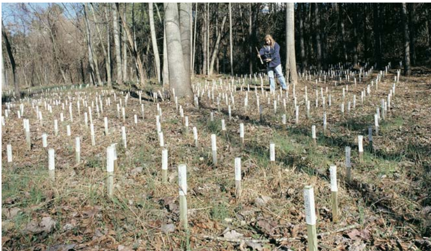
Continuous in-ground stake testing of traditional CCA lumber goes back 70 years. Newer formulations are holding up under similar testing, but some have only a four-year to 10-year track record.
