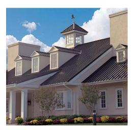
**Snap-On.** Standing seam roofing can be difficult to install without a trained metalworker on site. Petersen Aluminum is trying to change that with its *Snap-Clad* panels, which come with notched eaves, ready to install right out of the box. Held down by a hidden fastener system that allows for thermal expansion, Snap-Clad panels carry a UL-90 classification (meaning they can withstand winds of up to 188 mph). They come in a multitude of colors and sizes.
