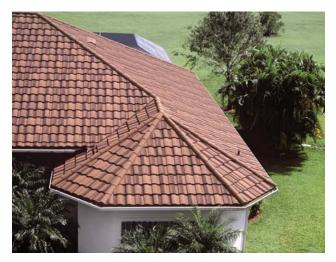
Quick Tile Panels. Adding a tile roofing system often requires structural reinforcement and a lengthy installation. To simplify the process, Metro Roof Products has released a lightweight roof panel with a classic Roman tile profile. Mounted on a 50-inch-by-16-inch sheet of 26-gauge galvanized steel, this product weighs only 1.5 pounds a square foot. It comes in various standard and premium colors and costs \$214 a square.
