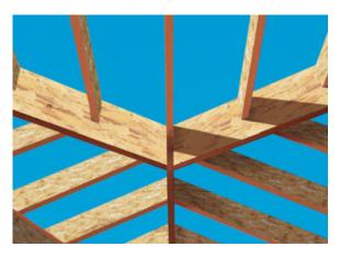
High-E Beams. LP's newest *SolidStart LSL* engineered lumber has a stiffness rating of 1.75E — the highest in the industry, says the maker. That means you can use an LSL beam or header for some spans that previously required a more expensive LVL. The products come in common dimensions in lengths of up to 64 feet; a 1<sup>3</sup>/4-inch-by-11<sup>1</sup>/4-inch LSL costs about \$3.50 per linear foot.
