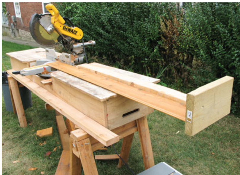
Figure 9. While the slats of many fences are run long and cut in place, in this instance they were to be of uniform length. A miter saw with a stop table sped the cutting.
