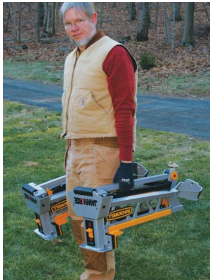
Figure 2. Folded up, the rear leg serves as a handle for toting the 45-pound JawHorses.
