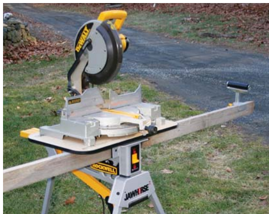
Figure 5. An optional miter-saw station works with an owner-supplied 2x4, which allows the outfeed rollers to be positioned wherever they'll work best.
