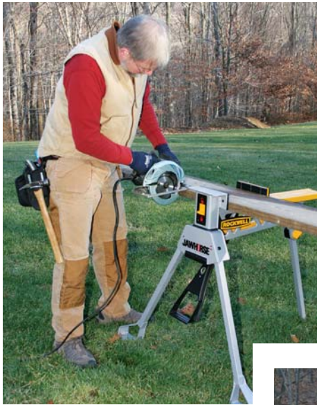
Figure 1. The JawHorses' stable tripod configuration and stout clamping mechanism securely support heavy deck materials.
