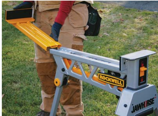
Figure 4. The jaw is easily reversed, increasing the stock clamping width to 37 inches.
