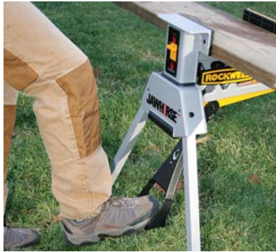
Figure 3. A foot pedal tightens the jaws, and the yellow tab at the front of the JawHorse locks the tightened jaws in place.
