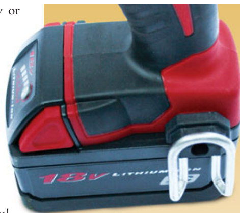
Figure 6. All the belt hooks are sturdy and made of metal, except the one on the Hitachi WH18DL.
