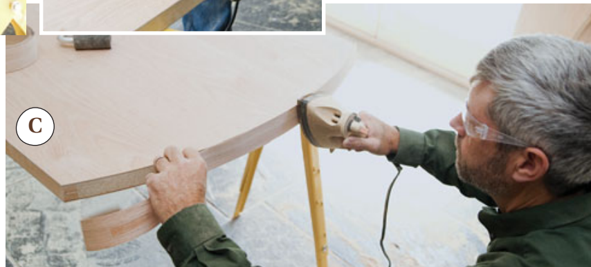
Figure 2. The author cuts segmented arch tops in solid-core door slabs with a router mounted on a trammel arm (A). After smoothing the cut with a belt sander (B), he irons on 1½- or 2-inch-wide veneer edge banding (C), which he trims to fit. The edge banding seals the top of the door.
