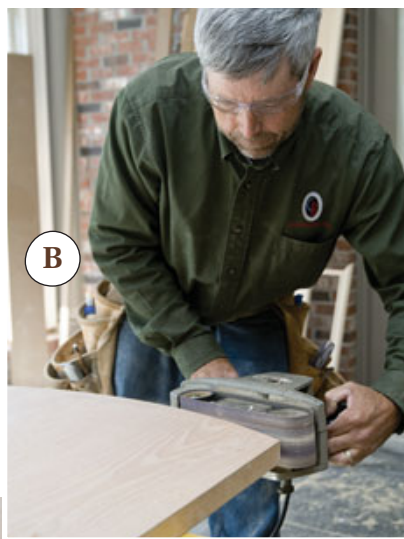
Figure 2. The author cuts segmented arch tops in solid-core door slabs with a router mounted on a trammel arm (A). After smoothing the cut with a belt sander (B), he irons on 1½- or 2-inch-wide veneer edge banding (C), which he trims to fit. The edge banding seals the top of the door.
