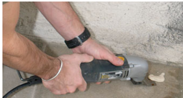
Figure 6. The versatile Rockwell SoniCrafter uses various vibrating blades for tasks ranging from plunge-cutting to cleaning up spilled construction adhesive to sanding.
