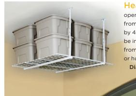
**Headroom.** HyLoft ceiling storage units take advantage of the open space beneath tall garage ceilings and come in a range of sizes from 3 by 3 feet to 4 by 8 feet. The *Model 540* pictured measures 45 by 45 inches and holds a maximum of 250 pounds; multiple units can be interconnected for more storage space. Heights can be adjusted from 16 to 28 inches so that units can be installed above garage doors or hung from sloped ceilings. Each unit costs about \$60.
