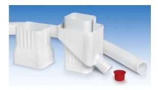
Simple Diversion. Oatey's Mystic Rainwater Collection System captures water from downspouts and redirects it through a tube into a rain barrel, which is not included. (Sealed rain barrels work best; common vented ones may overflow.) Leaves and sediment simply pass through the device, which can be attached to a downspout without removing the spout from the wall. The diverter costs \$20.
