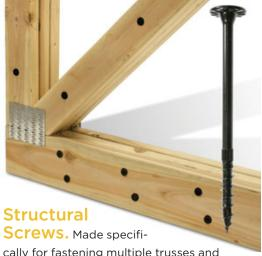
cally for fastening multiple trusses and engineered-wood assemblies, Strong-Drive SDW screws can be used to join up to four plies of 2-by or  $1^3$ /4-inch-thick materials. Fastening can be done from one side of the assembly, which eliminates a lot of heavy lifting. The screws have a large, flat head and a partial-thread design that draws materials together tightly. They come in eight lengths from  $2^7$ /8 to  $6^3$ /4 inches and cost \$30 to \$90 for a box of 50.
