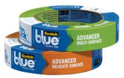
Sticky Edges. 3M's latest masking tape, ScotchBlue Advanced, has a moisture-activated additive that reacts with the water in latex paint to better seal along the tape edge. Since the adhesive treatment can't be rinsed or scraped off the tape, the rolls require no special handling, says the company. The tape comes in multi-surface and delicate-surface versions starting at about \$5 a roll.
