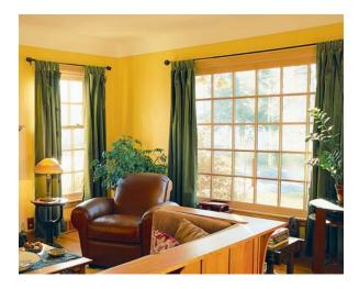
Fully Framed. Sold in three sill angles, Custom Shield replacement windows — double-hung, casement, awning, and direct-set units — come assembled in 3½-inch jambs for fast and easy installation. Options include several types of glazing, blind-stop covers, Z-trim, and interior prefinishing in 55 standard colors.
