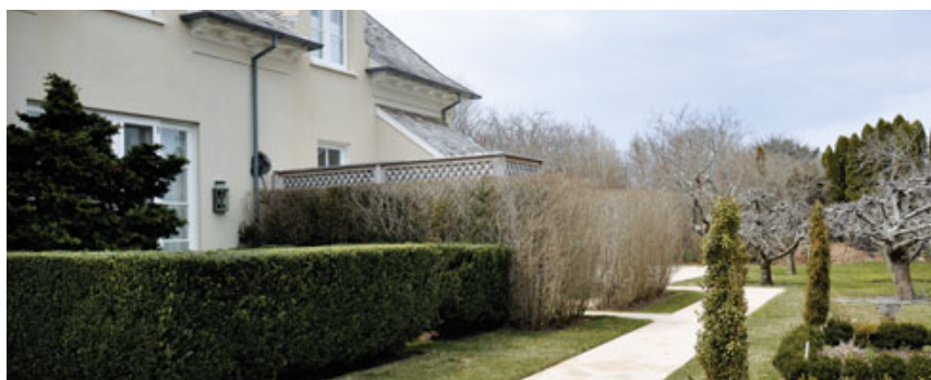
Figure 2. This 10-foot-tall barrier will provide almost twice the noise reduction of a 5-foot-tall barrier, even with clearances between the generator and enclosure limited because of the existing landscape design and zoning constraints.
