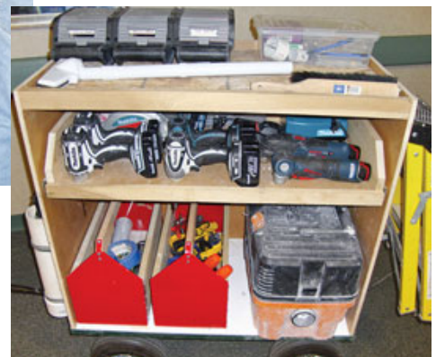
Figure 2. To work more efficiently, the crew used compact job carts customized for specific tasks, including a modified Sears service cart for demo, patching, and painting (above left) and a cabinet installation wagon compact enough to fit into an elevator (above right). The latter had a full-extension drawer containing a half-dozen cordless tools and their chargers and accessories (right).
