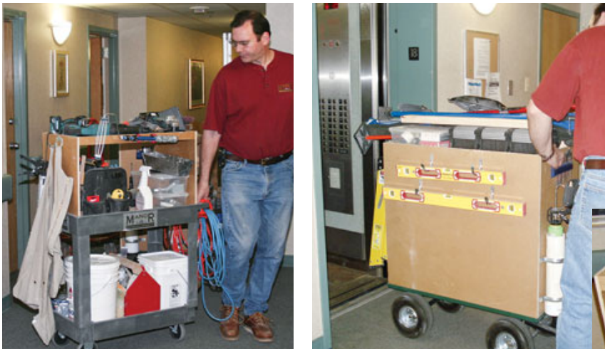
Figure 2. To work more efficiently, the crew used compact job carts customized for specific tasks, including a modified Sears service cart for demo, patching, and painting (above left) and a cabinet installation wagon compact enough to fit into an elevator (above right). The latter had a full-extension drawer containing a half-dozen cordless tools and their chargers and accessories (right).
