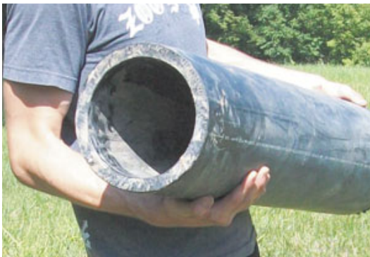
Figure 2. The heavy-duty HDPE pipe used in trenchless excavation has thick walls to withstand the tensile stress of pulling the pipe into an undersized borehole.
