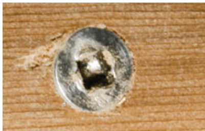
Figure 5. Square-drive, stainless-steel screws were a chore to drive because the driver bits constantly cammed out, which trashed bits and left sharp burrs on the screw heads (left). Star-drive screws didn't have that problem (right).
