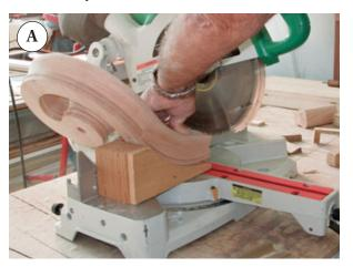
My shoe is laminated from several pieces of ½-inch birch plywood with a 9½-inch radius cut out of them with a router and trammel (B). I make the blanks slightly long. After gluing the stack together, I set the shoe on the miter saw and trim it at the 90-degree tangent point. Then, when the easing is in the shoe and the miter saw blade is registered against the tangent point, the resulting cut will be perfectly perpendicular.
