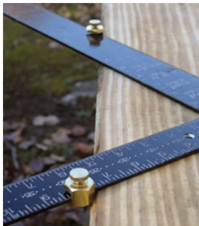
Figure 3. Stair nuts used on a framing square can be handy for marking out risers and treads, but stringer wane and eased edges make them difficult to use accurately.
