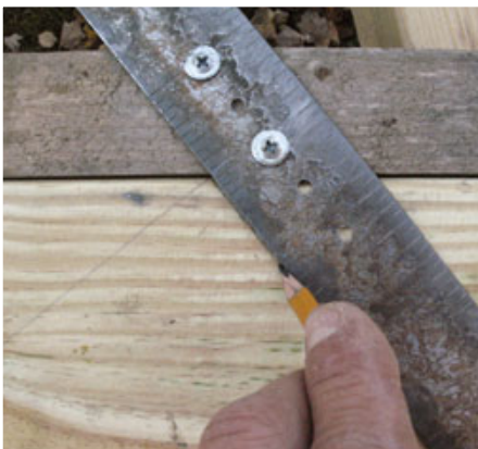
Figure 4. Rather than use stair nuts for marking out stringers, the author prefers to screw a straight 1x2 to a framing square. The 1x2 bridges any wane or other edge defects and provides a straight line that makes it easy to pinpoint riser and tread points when stepping off the stairs.
