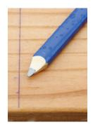
Wet/Dry Pencils • Sola, an Austrian company that makes high-end spirit levels, had a 9<sup>1</sup>/2-inch-long wet/dry carpenter pencil — the *KB* 24 — on display at its booth. I drew some lines and scribbled on a wet 2-by with both it and a normal carpenter pencil. The KB 24 made a darker blue line that didn't rub off. Lines made by the two pencils on a dry 2x4 were almost indistinguishable. The KB 24 currently costs \$1.25 at fastoolnow.com; a 13-pack is \$20 at sears.com.
