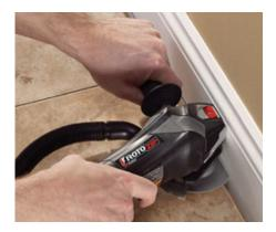
**Versatile Cutoff Saw** • The 7-amp RotoZip *ZipSaw* is a cross between a flushcut saw and an angle grinder, and it accepts RotoZip wheels or standard 4-inch grinder wheels. You can use it for everything from cutting curved notches in tile to flush-cutting a door jamb to accommodate new flooring. The saw lists for \$100 and includes a dust-collection kit and two wheels.
