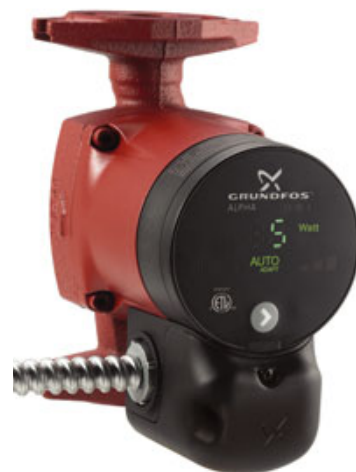
Figure 5. The newest generation of “smart” hydronic circulators uses ECM motors and microprocessor controls to regulate pressure in the system, greatly reducing electrical power requirements. The model shown is from Grundfos; similar circulators are available from Wilo, Bell & Gossett, and Taco.
