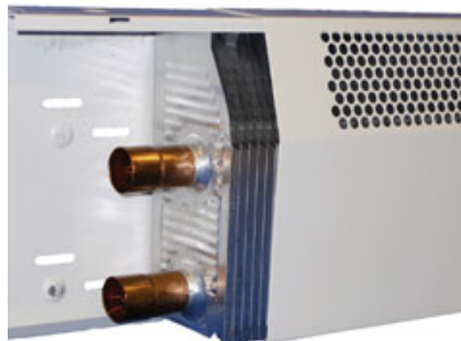
Figure 2. Smith Environmental's high-output fin-tube baseboard convector (left) uses parallel piping and closely spaced copper fins to deliver 400 Btu/hr per foot of length, with a water temperature of only 110°F. Jaga North America's panel radiator (below left and right) is enhanced with low-voltage micro-fans and can operate at water temperatures as low as 95°F.
